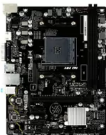
Placa Mae Biostar B450MHP, DDR4, Socket AM4, M-ATX, Chipset AMD B450, B450MHP
